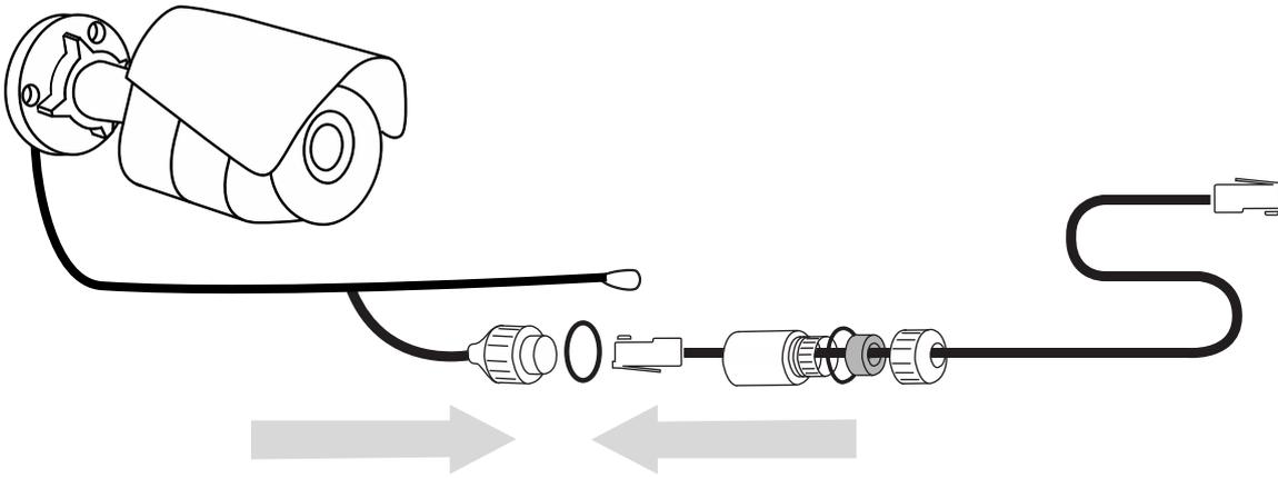
4. Connect the Camera to the Power Adapter and use the Power Cable Sealing Cover to secure the power plugs. Power on the Camera and verify the internet connection.
